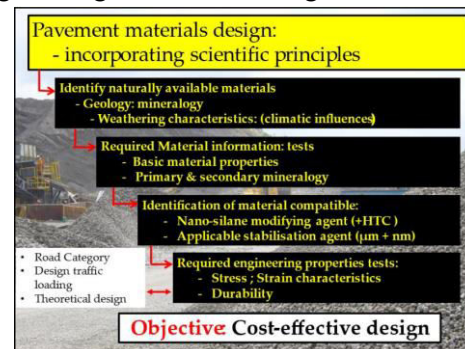
Figure 1: Recommended basic approach to road pavement materials design incorporating scientifically based concepts, developed for the selection of a material material compatible Newage (Nano) Modified Emulsion (NME) stabilising agent addressing the engineering requirements (physics) of a road pavement structure
